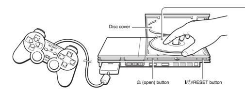
Place the disc in the console with the label side facing up.
